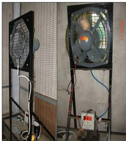
**Fig. 1:** Fan-Fogger system consisted of a blower with a copper ring having fine foggers (5 in no.) connected with a water tank through a high pressure pipe along the width wise of the pen
